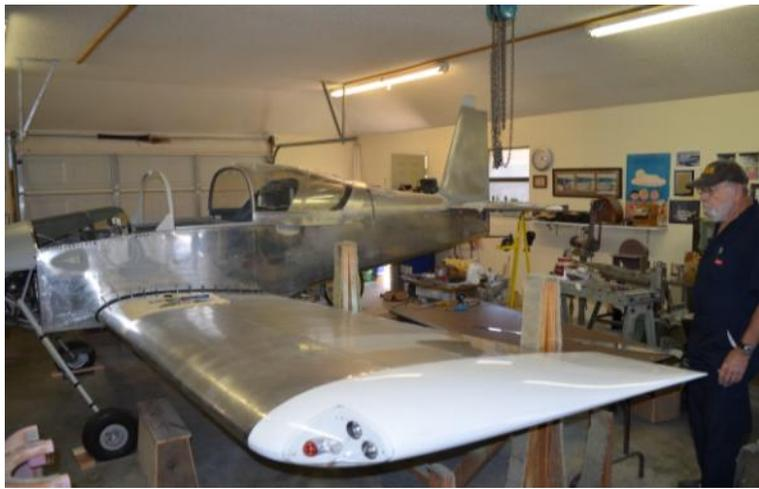
**Seth Hancock's** latest project is an RV-7 which, as can be seen in the left-hand photo, fills his garage. The –7 is one of many airplanes Seth has built., which aircraft include an RV-6, RV-8A and a Veri EZ. He still owns and flies the –8A. In the lower left image, Seth is shown installing the right wing-root fairing.
