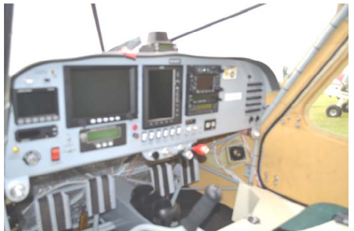
Bob Falstad who Also lives in Cross Country Estates spent time describing in detail the full panel in the Glaser he built. It houses ;a Grand Rapids EFIS, auto pilot, engine monitor and other devices that enhance the safety and precision of flight.
